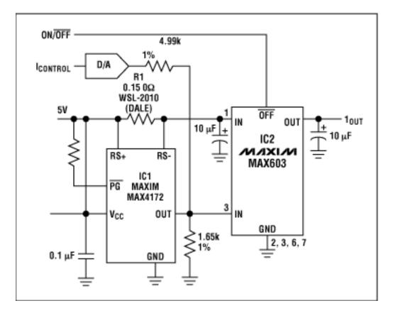
Figure 11. A variable, linear current source (MAX4173)
