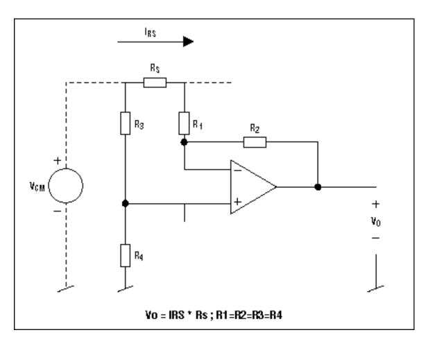
Figure 4. The differential amplifier is a basic component in high-side current measurements.
