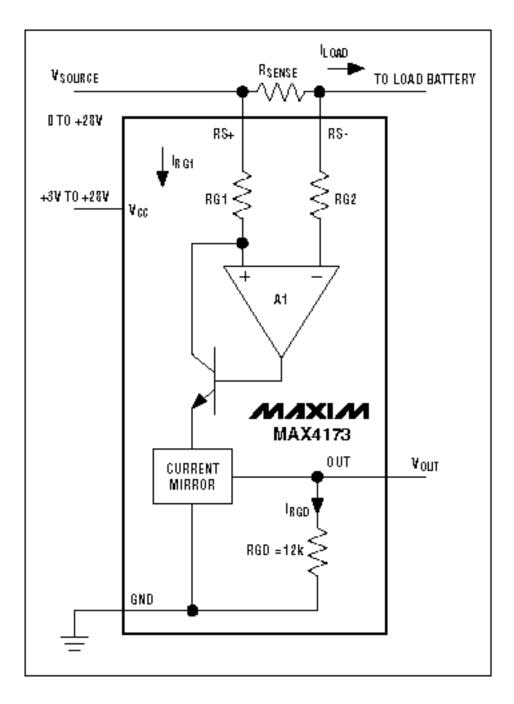
Figure 9. Yet another architecture for the unidirectional high-side current monitor (MAX4173)
