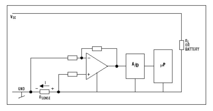
Figure 1. Principle of the low-side current monitor
