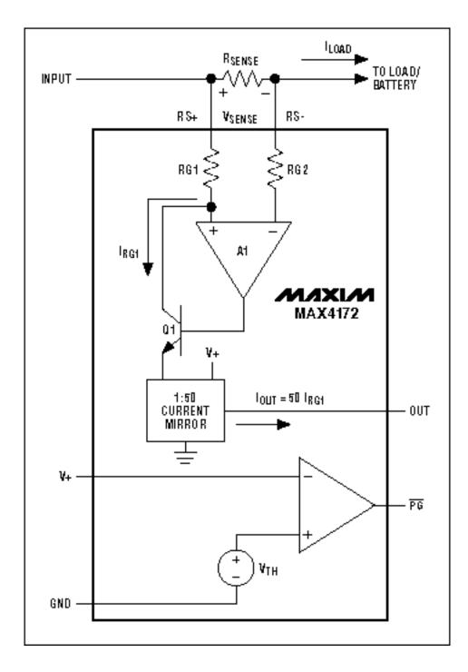
Figure 8. Another unidirectional high-side current monitor (MAX4172)
