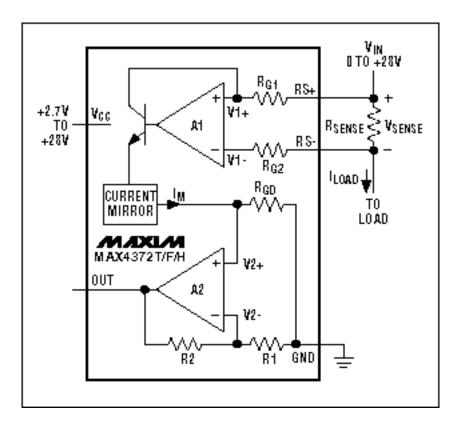
Figure 7. A unidirectional high-side current monitor (MAX4372)
